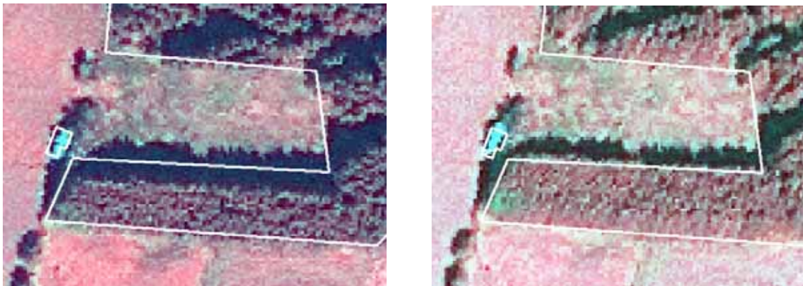
Figure 2. Error due to the parallax on the two elements from the stereo IKONOS pair. The viewing elevation angle was 71 degrees of the left image and 60 degrees on the right image.
