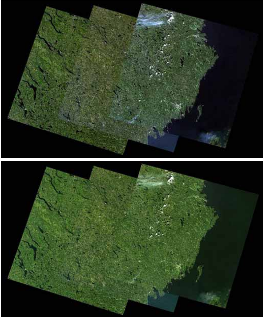
Figure 5. Mosaic of the visible bands in three Landsat scenes before (upper image ) and after calibration (lower image) The left scene was registered July 27, 2000, the middle scene in August 11, 2002 and the right scene in July 27, 2000.
