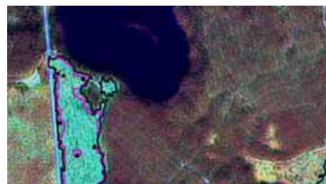
Figure 5. Mapping from SWIR single band difference image between 2.5 m resolution merged SPOT-5 2002 and Landsat-7 ETM+ 1999 scenes.
