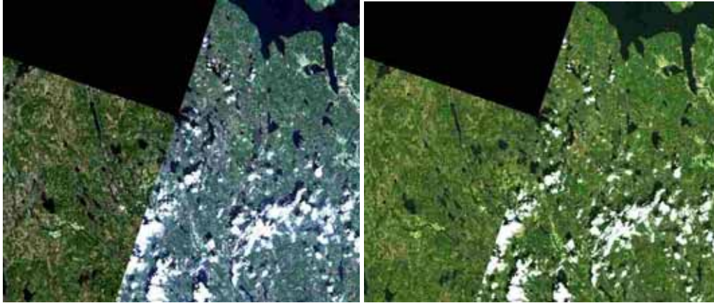
Figure 1. Results of relative calibration of Landsat imagery against the MODIS BRDF-corrected surface reflectance product. The left image shows the uncorrected scenes (top of atmosphere radiance) and the result after correction is shown in the right image. Local variations in atmospheric optical thickness and illumination effects due to sloping terrain in the Landsat data has been removed by processing in the MUNIN production line.
